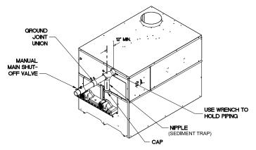
Figure 28 – Gas Line Connection
